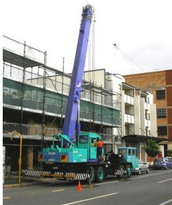
Figure 2 – Hazard striping on a mobile crane
