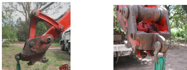
Figure 7 and Figure 8 - Lifting attachment with a closed eye on excavator
