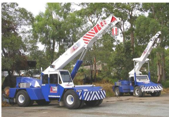
Figure 5 – Pick-and-carry mobile cranes (non-slewing hydraulic cranes)
