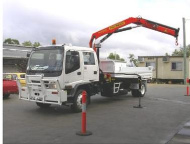
Figure 9 – Vehicle-loading crane
