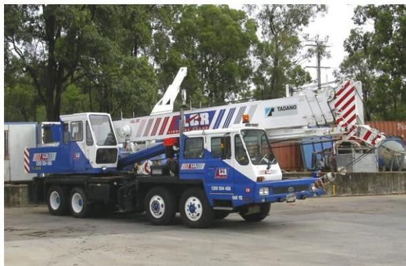
Figure 1 – Hydraulic slewing mobile crane
