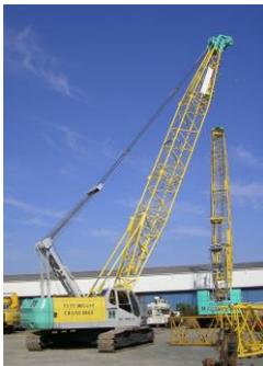
*Figure 6 – Lattice boom crawler crane*
