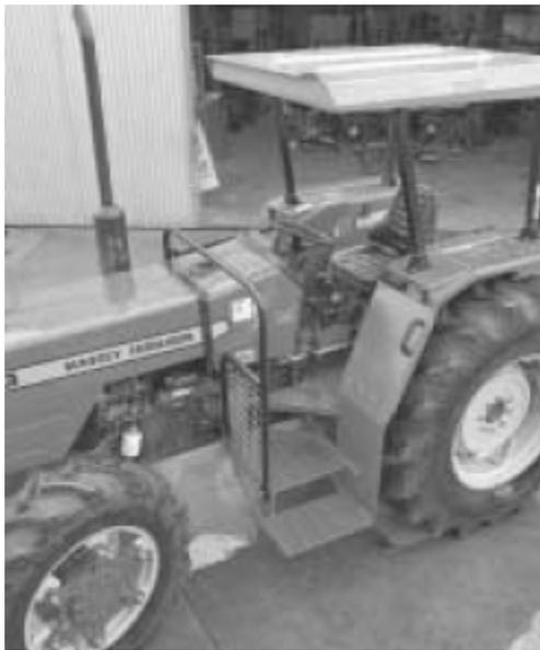
*A safe means for access and exit has been fitted to this tractor.*
